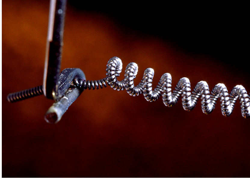
Figure 1: The coiled coil of an incandescent bulb filament.
