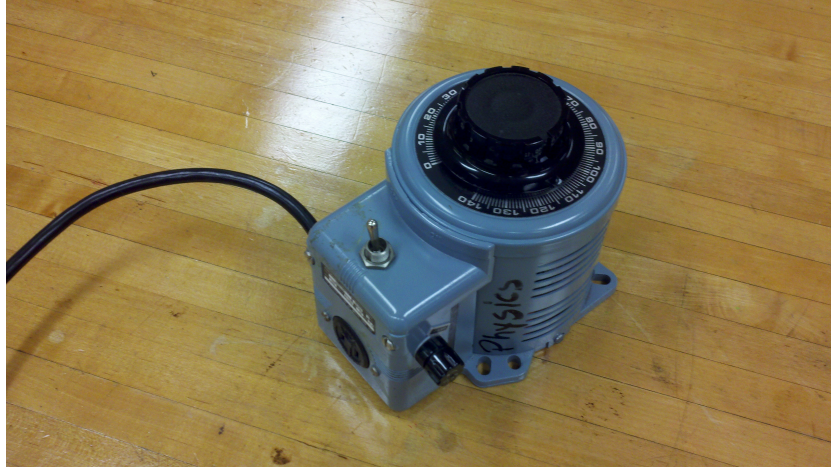
Figure 2: The variable transformer, aka variac.
