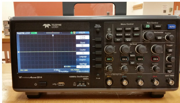
Figure 2: The front panel of the WaveAce 2014 Digital Oscilloscope.
